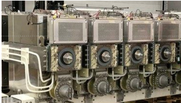
Figure 6 (a) Half Bridge Converter Cells
