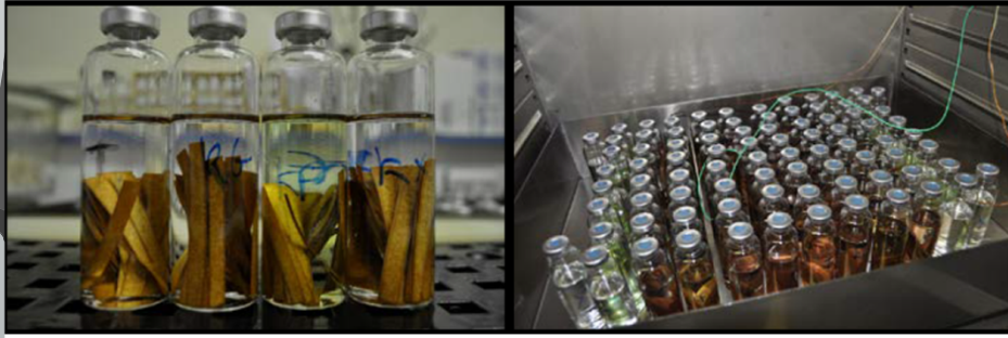
Figure 1: Ageing of sealed vials filled with insulating liquid and Kraft paper
