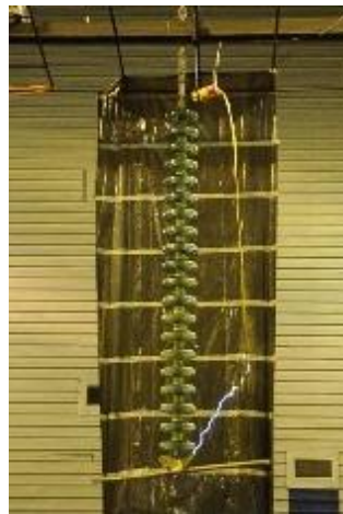
Figure 6: Flashover observed at 30 cm away from the string (NETFA Lab)
